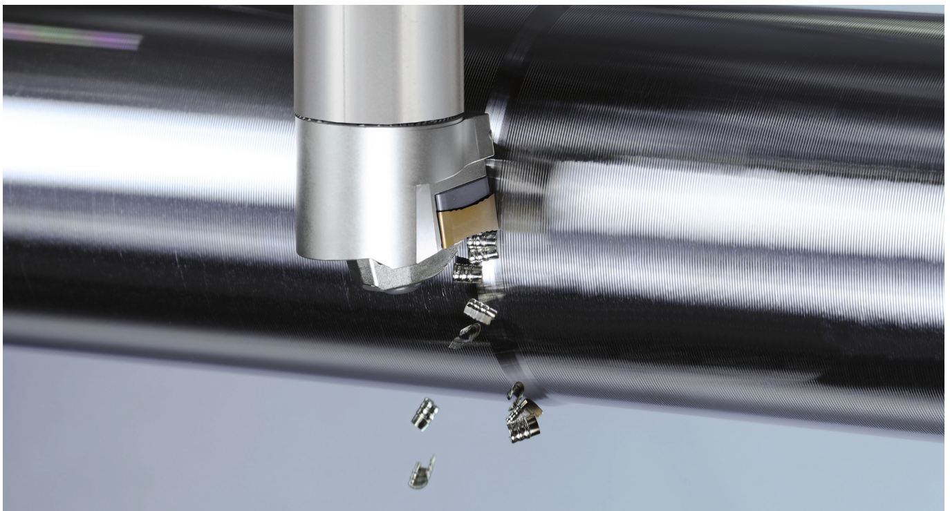
Y-axis turning means chips fall to the ground thus avoiding collision with the workpiece
