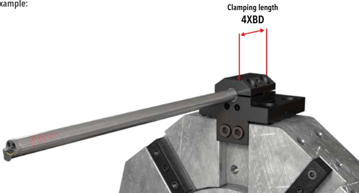
b.) Flat-bed lathe with a tool post provides higher rigidity compared to turret clamping. When using larger diameter bars, the moment exerted on the clamping tool (just by the bars weight) is increased dramatically.
