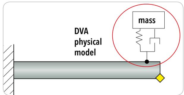
A mechanism is designed to preload the elastomers and therefore to modify the stiffness of their equivalent spring. Modification of the spring stiffness causes a change of the DVA natural frequency. The DVA system is tuned such that its natural frequency is brought close to that of the tool without DVA. This is done in order to introduce a phase shift between the tool and the DVA mass vibration, eventually causing attenuation of the oscillation amplitude of the tool.
