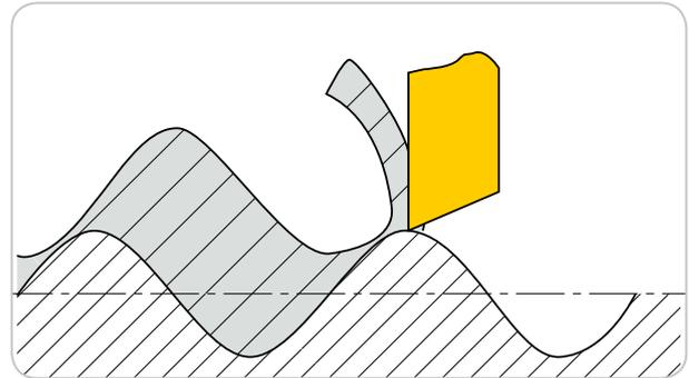
Chatter vibrations are detrimental to the safety and quality of machining operations. They cause a rough surface finish, increase cutting forces, reduce tool and machine life, decrease productivity, and create irritating high noises.
