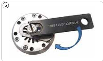
Fig. 34 a + b Inserting wrench
