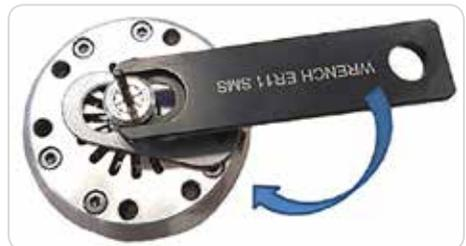
Fig. 9. HSM HPC Spindle with shaft lock mechanism
