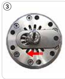
Fig. 33 a + b Inserting shaft lock flat key
