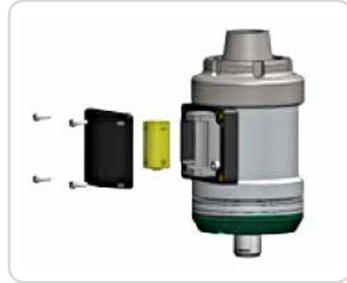
Fig. 12. Battery case opening
