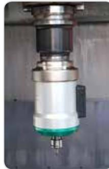
Fig. 28. HSM GreenJet Spindle on CNC machine
