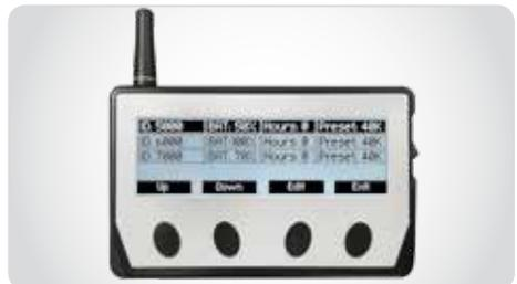
Fig. 21. Disconnection list on multiple signals screen
