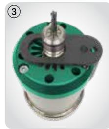
Fig. 34 Slide key into place
