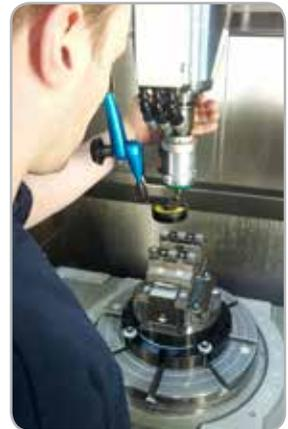
*Fig. 37. Manual runout testing*
