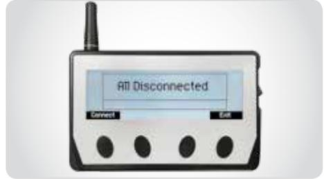
Fig. 22. Disconnect all sensors screen
