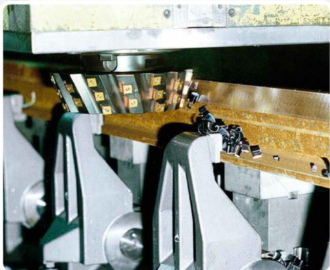
Tangential tool design for the most various machining operations and profiles.
