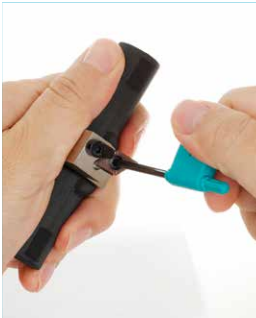
Modular heads for Y-axis (QE1Y...)
