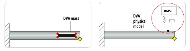
A mechanism is designed to preload the elastomers and therefore to modify the stiffness of their equivalent spring. Modification of the spring stiffness causes a change of the DVA natural frequency. The DVA system is tuned such that its natural frequency is brought close to that of the tool without DVA. This is done in order to introduce a phase shift between the tool and the DVA mass vibration, eventually causing attenuation of the oscillation amplitude of the tool.
