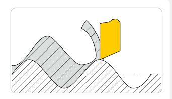
Chatter vibrations are detrimental to the safety and quality of machining operations. They cause a rough surface finish, increase cutting forces, reduce tool and machine life, decrease productivity, and create irritating high noises.
