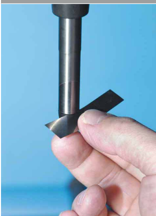
Fig. 4: the feeler gauge must NOT fit in the gap
