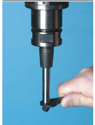
Fig. 3: tighten tip in the holder
