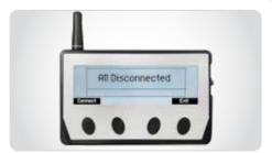
Fig. 22. Disconnect all sensors screen
