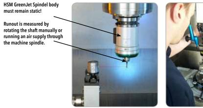
Fig. 36. Optical runout testing
