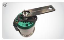
Fig. 35 Insert wrench into slots on nut - turn clockwise
