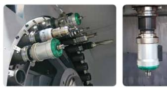
Fig. 28. HSM GreenJet Spindle on CNC machine
